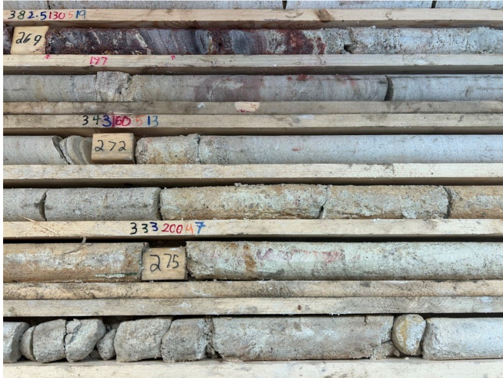
Figure 5 – Altered sandstone 17 to 35 metres above the unconformity in Target Area B (LE24-165, 269.7-288.1m). The core is strongly bleached with intervals of desilicification, strong clay alteration (mostly in the lower six rows) and local secondary hematite (some of the hematite in rows two to four). Mineral spectroscopy classifies the clay as 100% illite.
