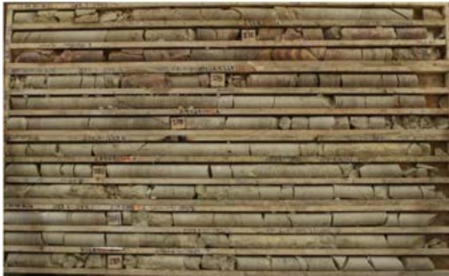
Figure 5 – Altered sandstone 17 to 35 metres above the unconformity in Target Area B (LE24-165, 269.7-288.1m). The core is strongly bleached with intervals of desilicification, strong clay alteration (mostly in the lower six rows) and local secondary hematite (some of the hematite in rows two to four). Mineral spectroscopy classifies the clay as 100% illite.
