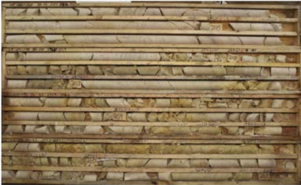
Figure 7 – Altered sandstone 10 to 30 metres above the unconformity in Target Area D (LE24-172, 260.7- 278.7m). The core is moderately to strongly bleached with patches of preserved purple diagenetic hematite. Much of the photographed interval is rubbly and desilicified, with local intervals of intense clay alteration and patchy secondary hematite. Mineral spectroscopy indicates an illite – dickite clay species mixture.
