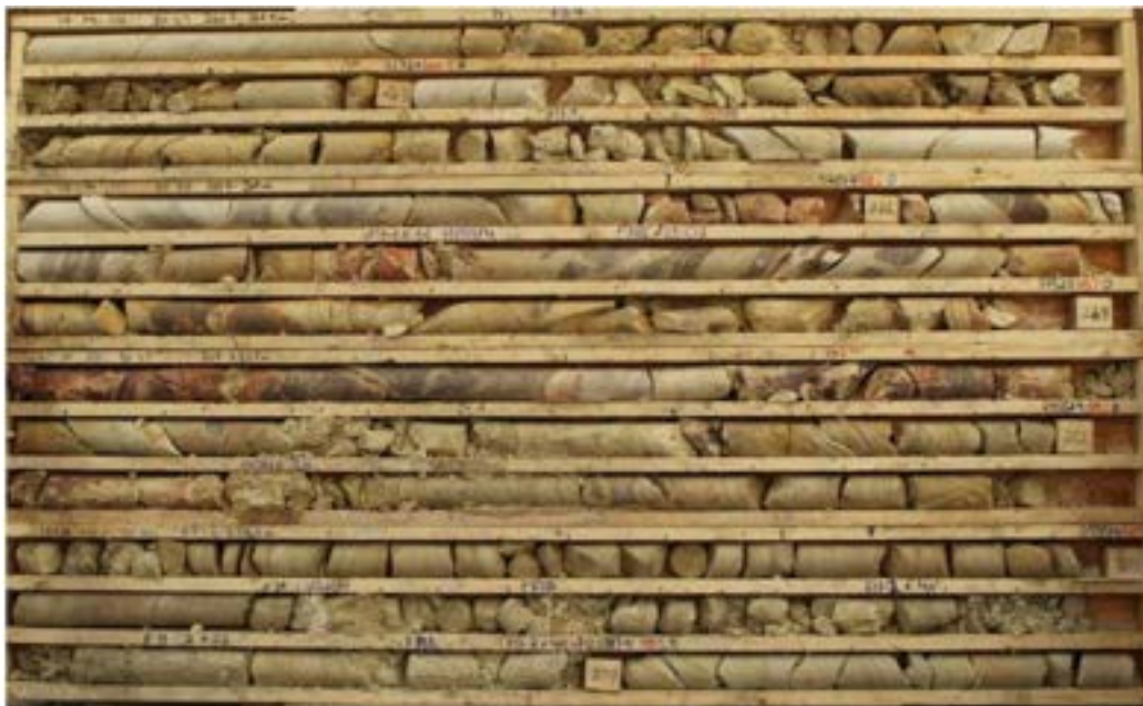
Figure 7 – Altered sandstone 10 to 30 metres above the unconformity in Target Area D (LE24-172, 260.7- 278.7m). The core is moderately to strongly bleached with patches of preserved purple diagenetic hematite. Much of the photographed interval is rubbly and desilicified, with local intervals of intense clay alteration and patchy secondary hematite. Mineral spectroscopy indicates an illite – dickite clay species mixture.
