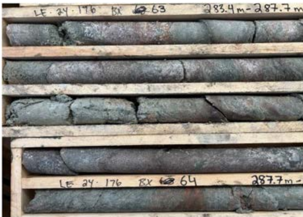
Figure 8 – Chloritized basement gneisses 5 to 10 metres below the unconformity in Target Area D (LE24-176, 283.4-289.5m). The mineral spectroscopy classification is dominated by sudoite (chlorite) with lesser illite.
