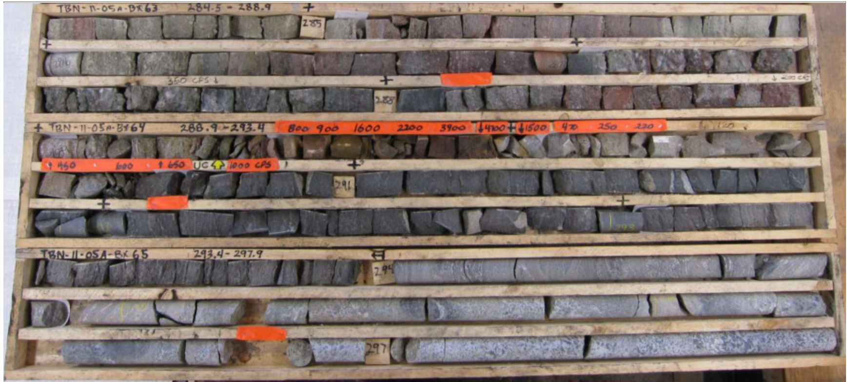
Figure 10-2: Drill Hole TBN-11-05A – Unconformity Intersection
